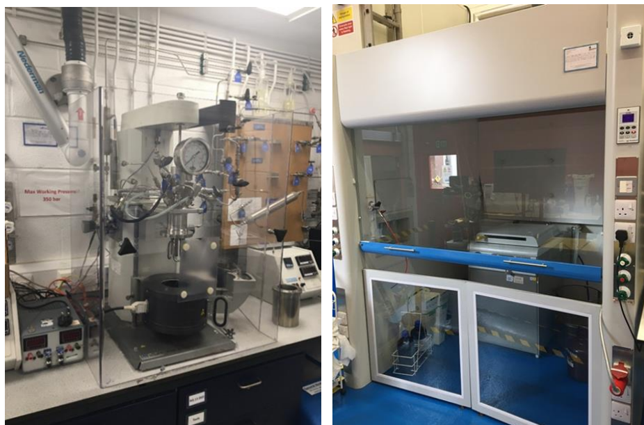
Figure 8 An example of LEV for bench-top equipment (left) and walk-in enclosure (right) (photo credit: Heriot-Watt University)
