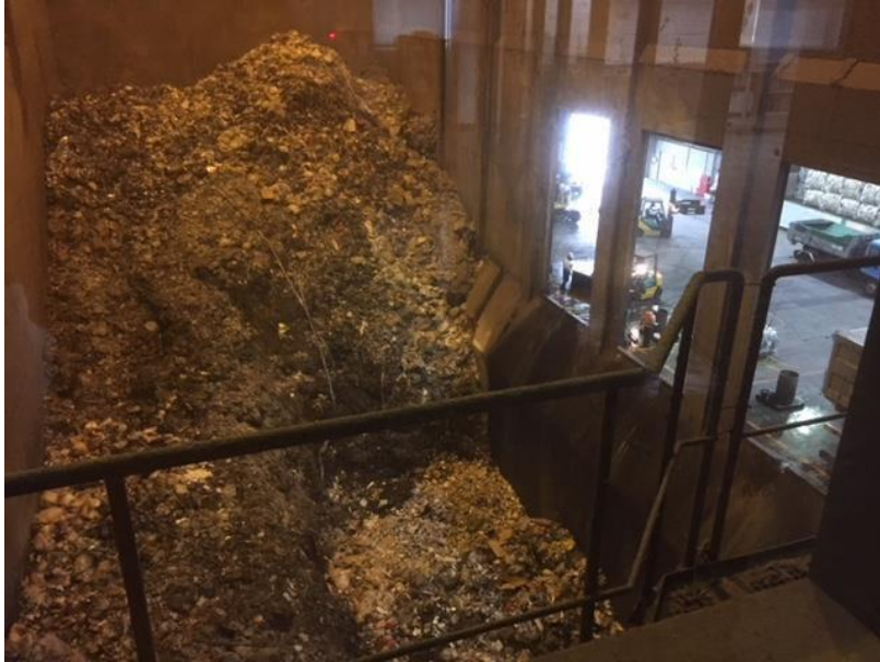
Unsorted non recycled, non-compostable municipal solid waste fed directly to gasifier and continuously converted to ethanol.
